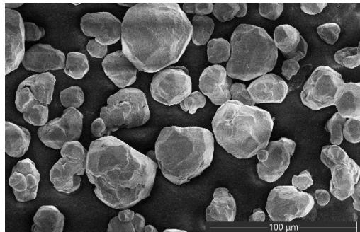
The material's 99.7% Fe purity and low impurity content support strong bonding, uniform coating structure, and reliable magnetic and thermal performance. This makes it well-suited for functional iron-based coatings and for repair or dimensional restoration of steel components.
